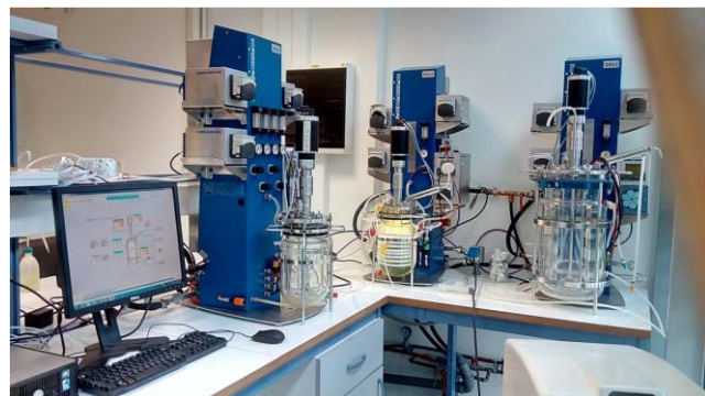
Bioreactors system (Bioengineering) - 2 L, 3,5 L and 15 L capacity
